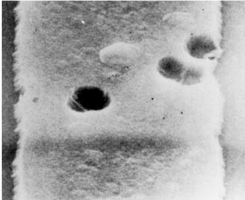
FIGURE 2077-18. (5,000X) General metallization voids (reject).
