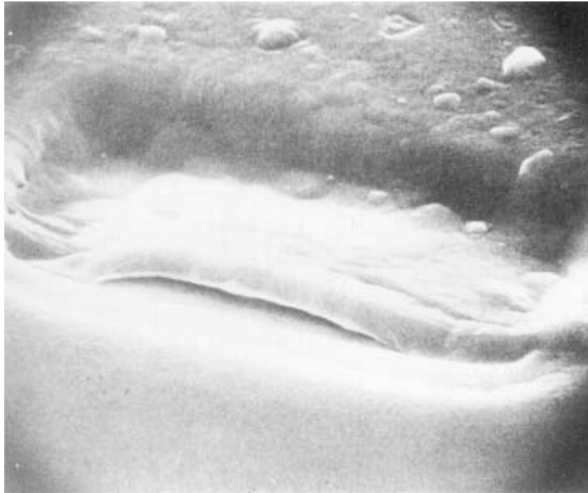
FIGURE 2077-16. (5,000X) Peeling or lifting of general metallization in contact window area (reject).
