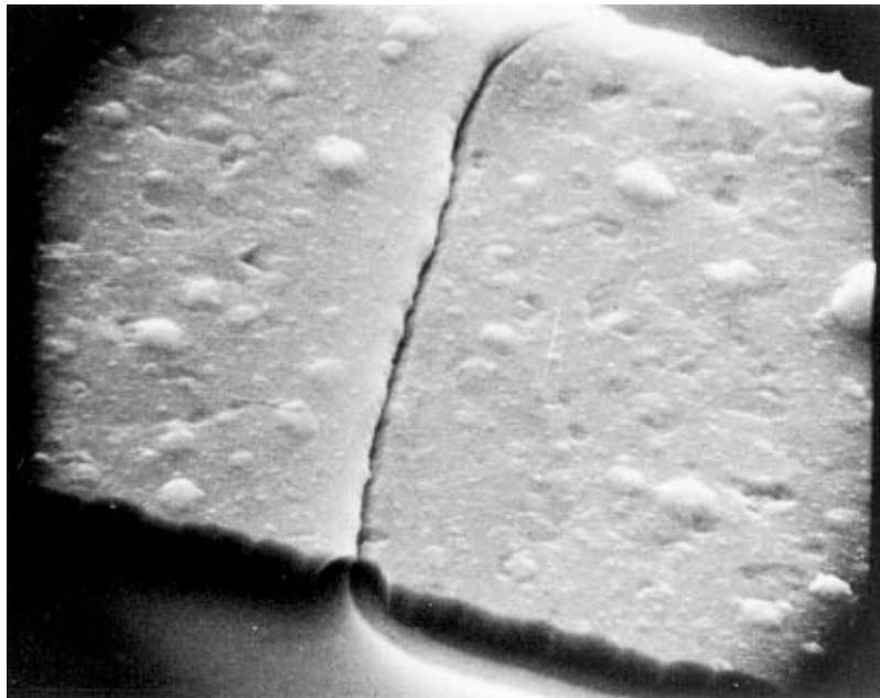
FIGURE 2077-7. (5,000X) Tunnel/cave at oxide step (reject).
